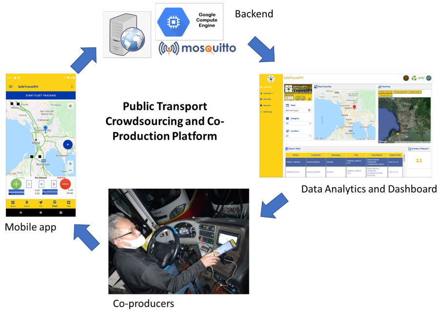
Figure 6. Structure of SafeTravelPH app and platform
