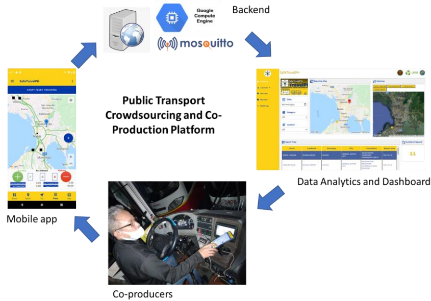
Figure 8. Structure of SafeTravelPH app and platform architecture
