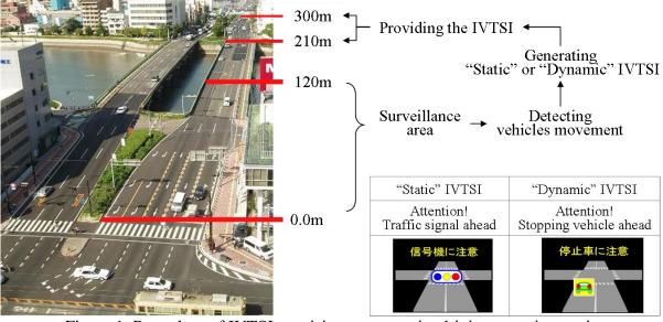
Figure 1. Procedure of IVTSI provision at an on-site driving experiment site
