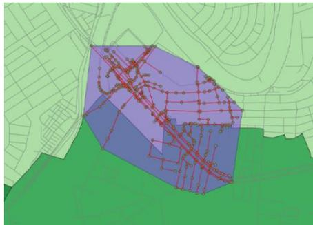
Figure 3-1. QGIS Network Analysis Service Area Sample Output
