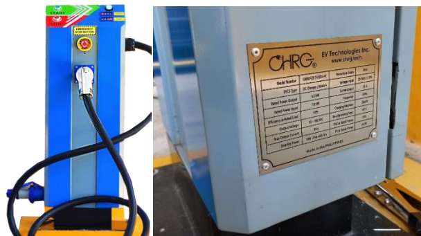
Figure 9: DC Fast Charger with nameplate
