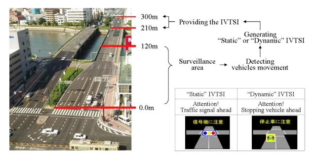
Figure 1. Procedure of IVTSI provision at an on-site driving experiment site
