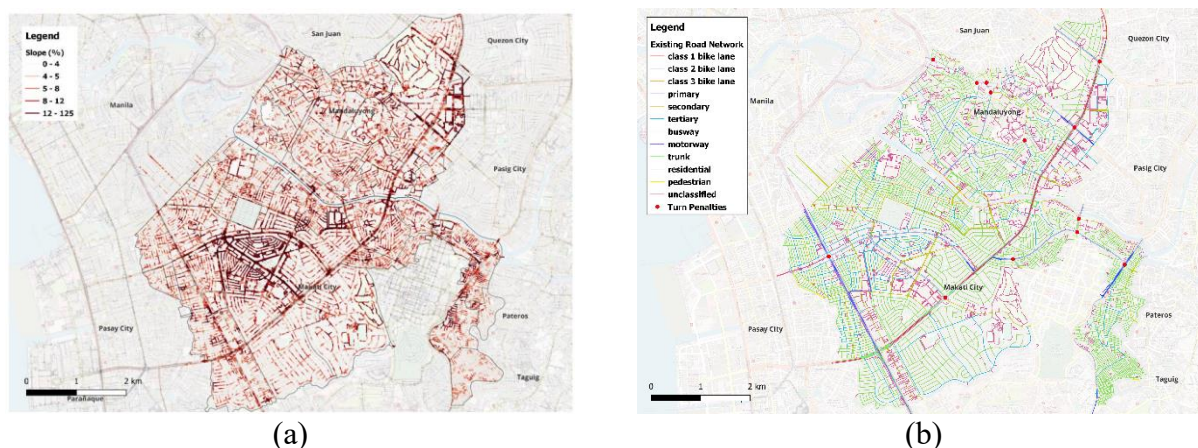
Figure 2. Network map of (a) slope percentage, (b) existing road classifications and turn penalties
